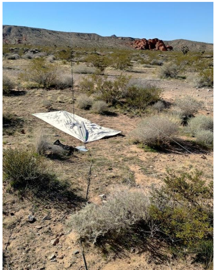
Fred's (KI7TPD) portable HF Ventenna Antenna setting on his Faraday blanket used as a ground plane.
