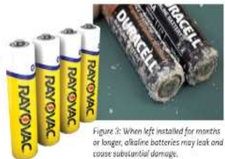
Figure 2: Heavy-duty batteries may look like alkaline cells, but their internal chemistry is quite different.
