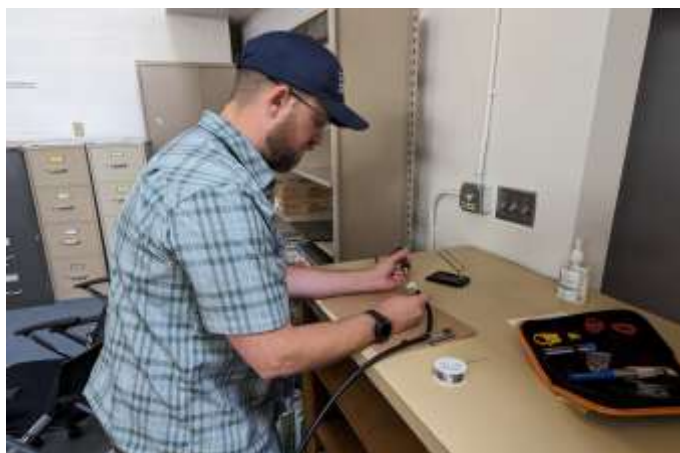
Mike (KI7ZXC) Soldering the connectors to the coax. Note: Not pictured were George (AL7BX) and Dennis (W6DLW).
