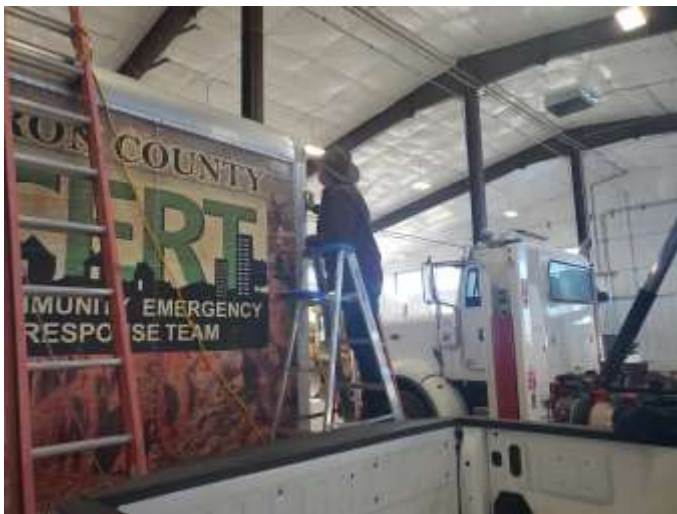
Fred (KI7TPD) inspecting seams prior to caulking
