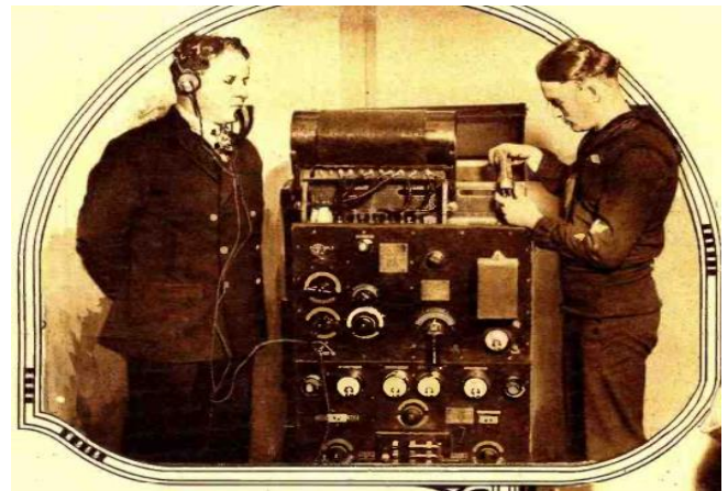
NEW NAVY TRANSMITTER with a power of 300 watts. It employs twelve 50-watt tubes and can be used for C.W., I.C.W. or Radiophone. It was designed especially for use on the Man-o-wars. Chief Gunner F. C. Nantz and John Cox are shown demonstrating it at the Radio World's Fair. © Kadel & Herbert.
