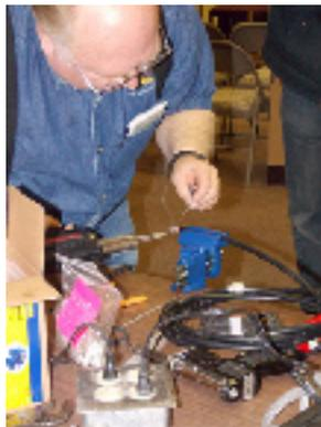
Dick shows how to solder the braid before inserting into the PL259 connector.
