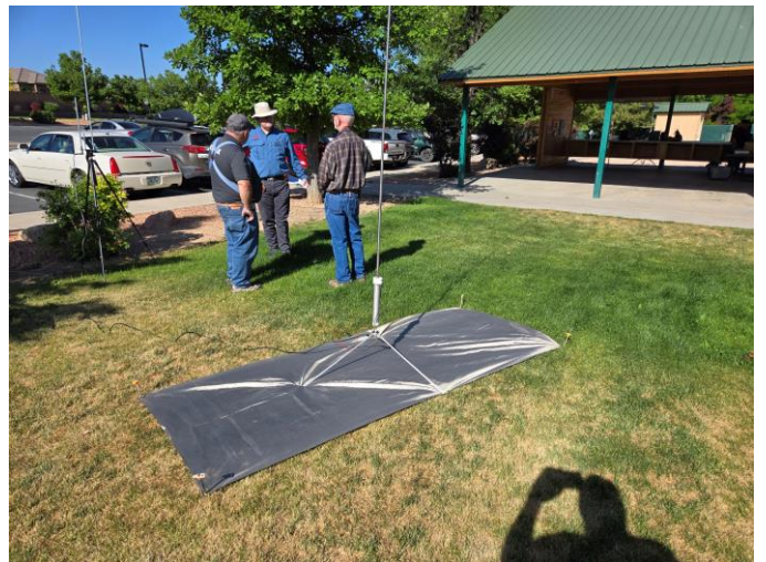
Ron (K7HDX) using a Faraday Cloth for a ground plane on the Wolf River 1000 HF antenna.
