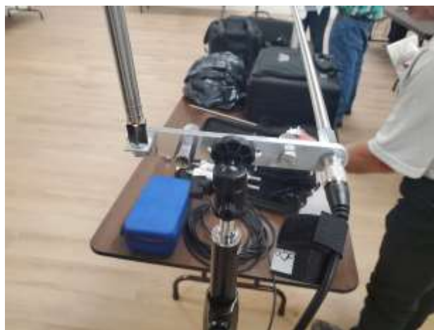
Close up of bracket use to make the different configurations using the telescoping whips.
