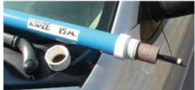
A completed travel tube for an antenna for 15 meters. (Bob Patterson, KSDZE, photo)
