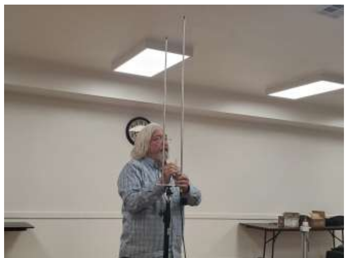
Jpole set up for 2 meter and 70 centimeters.
