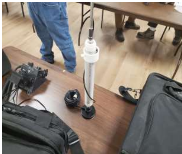
Wolf River 1000 Coil set up with a magmount for easy deployment.
