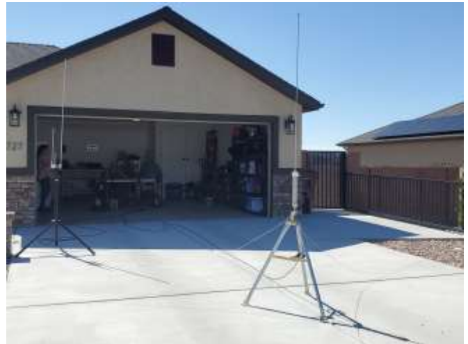
Wolf River Coil HF Antenna right foreground and the K&N Jpole Antenna to he left.
