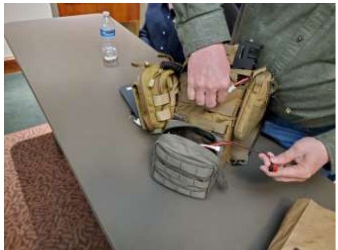
Another view of Ron's portable go kit. Showing where the battery cable is located and where they connect to the radio. The back of kit has a sleeve in back where is Tablet PC is stored for digital work.
