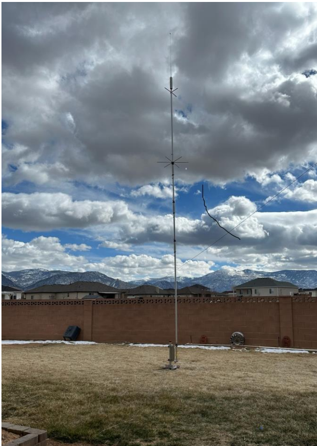
Antenna, Vertical, HF, 5-Band, 80, 40, 20, 15, 10 meters
