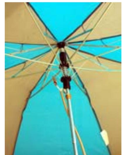
Ken's Umbrella Antenna with the center of coax clipped to a stringer and the ground attached to the metal hand shaft.
