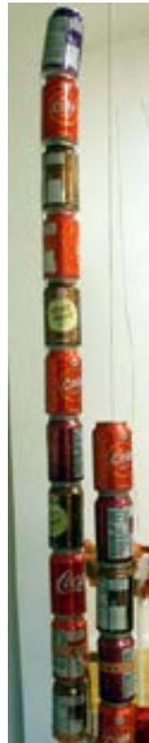
Left Side: Ken's aluminum can 2 meter antenna held together by string and gravity.
