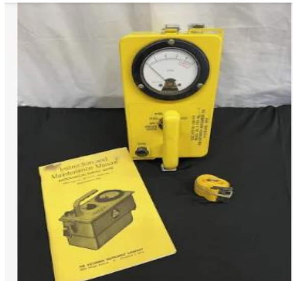
This is CDV 717 Radiation Meter. Most of the members of the unit have this meter.
