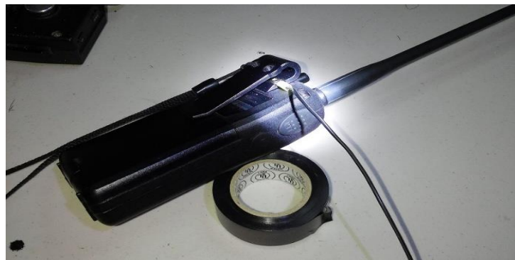
Photo above shows counterpoise wire connected to a screw on the back of the HT.
