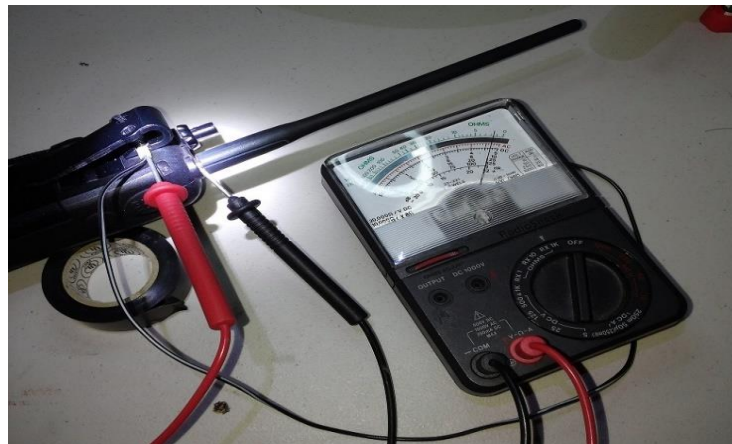
Checking continuity between screw and ground side of antenna. That's all there is to it. 73, K5LUO
